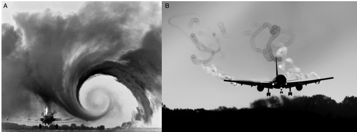
Fig. 1 Although flow structures in the air are usually difficult to visualize, they can be large, powerful, and long lasting, and have tremendous potential to influence the mechanics and aerodynamics of animal flight. (A) The air flow from the wing of this agricultural plane is made visible by a technique that uses colored smoke rising from the ground. The swirl at the wingtip traces the aircraft's wake vortex, which exerts a powerful influence on the flow field behind the plane. Photograph courtesy of NASA. (B) Wingtip vortices persist for many hundreds of times the distance from the leading to trailing edges, the chord length, of an airfoil, and can be perturbed by local air conditions such as small scale turbulence, as illustrated in this photograph of a landing Boeing 757 at London's Gatwick Airport. Photograph used with permission from AirTeamImages.com.
